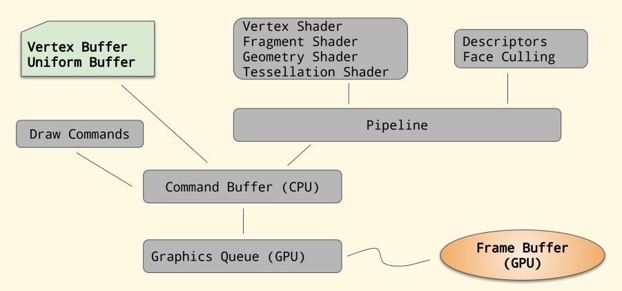
When the frame buffer is ready, a previously configured semaphore is triggered which presents the output
